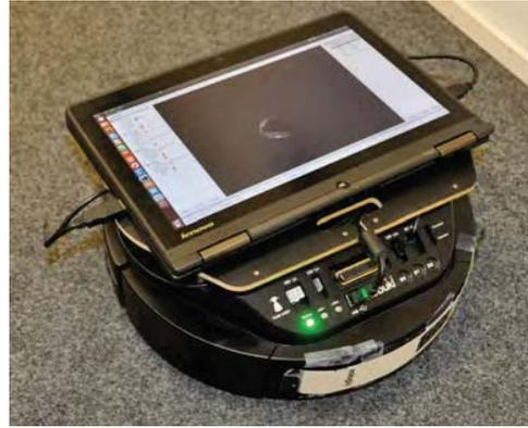
Fig. 4. Experimental setup comprising Kobuki robot and capacitive sensor.
