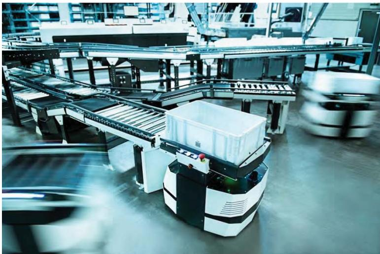
Smart Container Shuttle – the smaller of incubed IT's two standard shuttles
