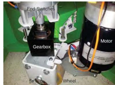
Fig. 2: Ackerman-steering of the forklift. Steering motor on top not shown.
