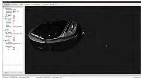
Fig. 5. Visualization of the sensor data in RVIZ. The blue dots depict the distance between the robot an object in front of the robot.
