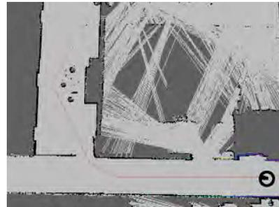
Fig. 4: Evaluation task. The figure shows the occupancy grid of the environment (gray) and a sample generated path (red).
