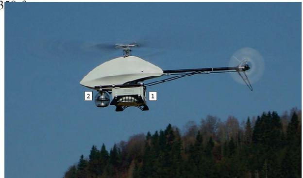
Fig. 2. Compact UAV equipped with roll-tilt compensated, multi-spectral imaging sensor (2) and data acquisition hardware (1).
