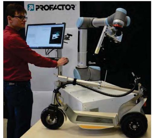
Figure 2: Universal Robot UR10 with mounted Kinect and an example work piece (here the UCARVER of GW St.Pölten Integrative Betriebe GmbH).
