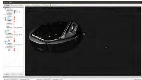
Fig. 5. Visualization of the sensor data in RVIZ. The blue dots depict the distance between the robot and an object.
