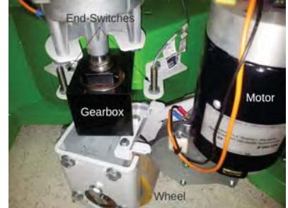
Fig. 2: Ackerman-steering of the forklift. Steering motor on top not shown.
