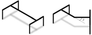
Fig. 1. Sketch of the possible different platforms and supports: on the left a classical wheeled system with a rigid frame, on the right an articulated platform with a  $\beta$  steering angle
