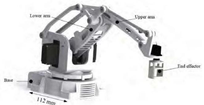
Figure 1: Robot 3D-Model rendered in SolidWorks.
