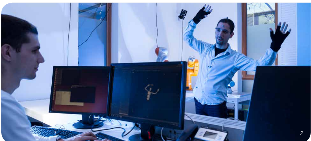
Photos: 1) Force and pressure measurement complying with ISO/TS 15066; 2) Optitrack – vision-based tracking system
