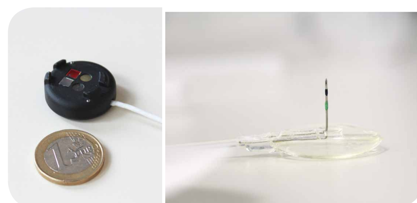
Fig. 3: left: SPIDIMAN glucose reader with 1 Euro coin for size comparison; right: Insulin infusion set with two sensors applied onto the needle
