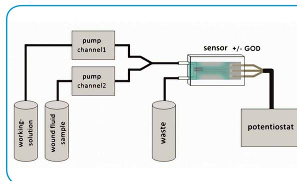
Figure 1: Scheme of the measurement system
