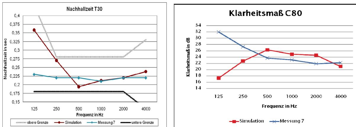
**Figure 2.** Reverberation time T30 (left) and Clarity C80 (right) of the equipped listening room (red – simulation, blue – measurement)
