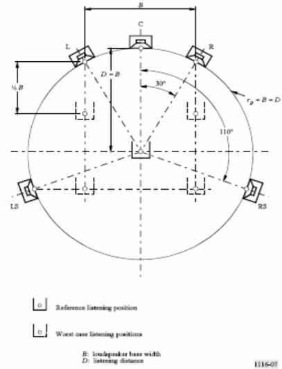
**Figure 3.** Listening room with acoustic absorbers, equipment and furniture (left); positioning of the loudspeakers according to the ITU standard's recommendation (right)
