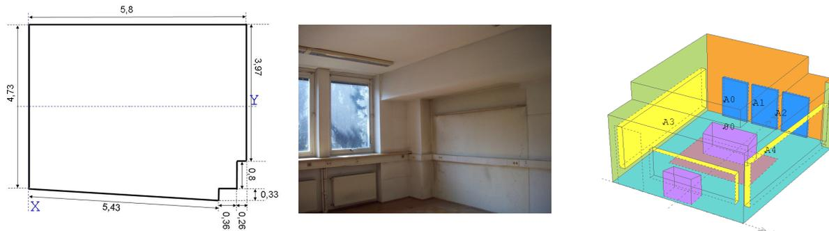
**Figure 1.** Ground plan and photo of the target room at JOANNEUM RESEARCH (left and middle), room model with absorbers and furniture implemented in CATT Acoustic® (right)
