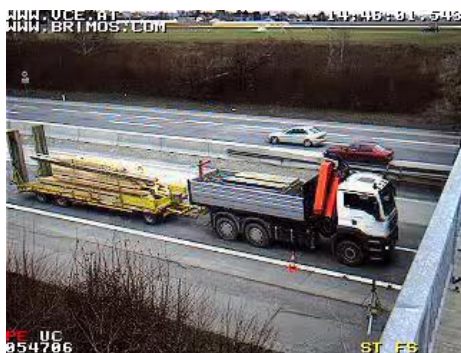
Fig.3 passing pattern of a triple axle lorry with a triple-axle trailer
