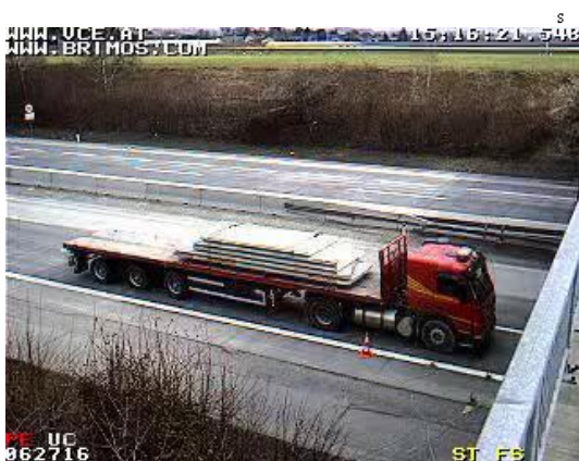
Fig. 5 passing pattern of an articulated lorry indicating the distribution of axle load
