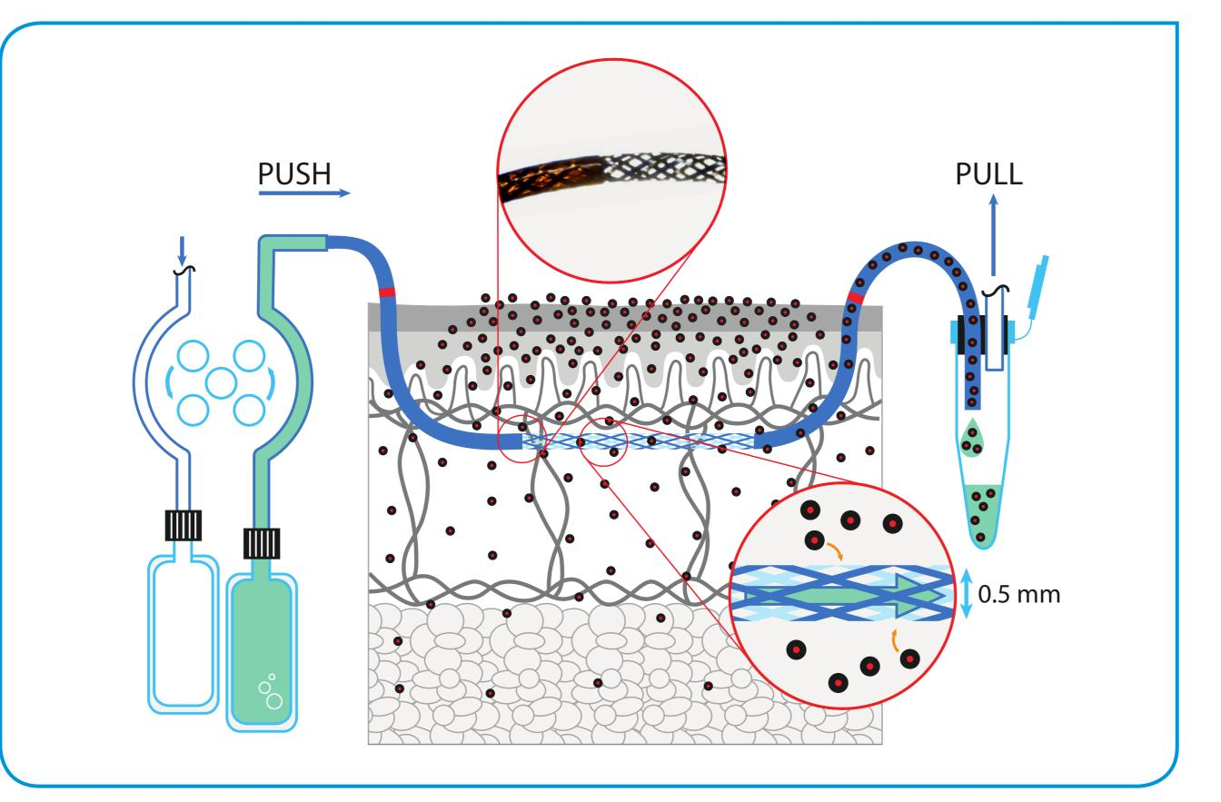
Figure 1: Open Flow Microperfusion (OFM). dOFM, a universal linear certified probe designed for dermal and abcutaneous use in humans, continuously delivers dermal interstitial fluid for the study of PK and PD in the target tissue. Continuous sample collection is controlled by a wearable pump. All devices are CE-certified for human use and were designed and patented by JOANNEUM RESEARCH, Graz, Austria
