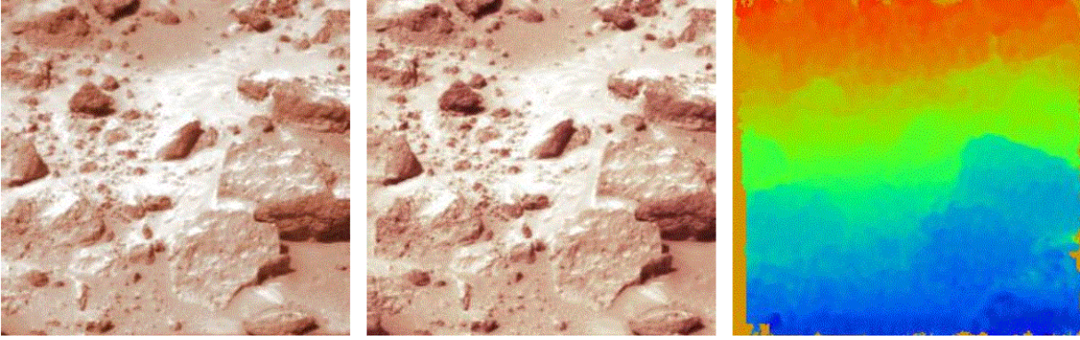
Figure 3. Left, center: Mars Pathfinder landing site stereo images. Right: HFVM Disparity image (false color)
