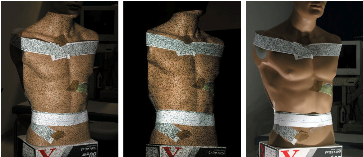
Figure 2: l : Input images of one sector (of eight). left and middle : Random pattern projected for left and right shape camera, right : Texture image. The target is a male dress doll, with some auxiliary target patterns glued on the surface (see also Figure 2).
