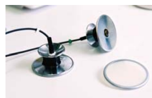
Figure 1: Newly developed sensors for picking up respiratory sounds; miniature microphones are integrated in the stethoscope head
