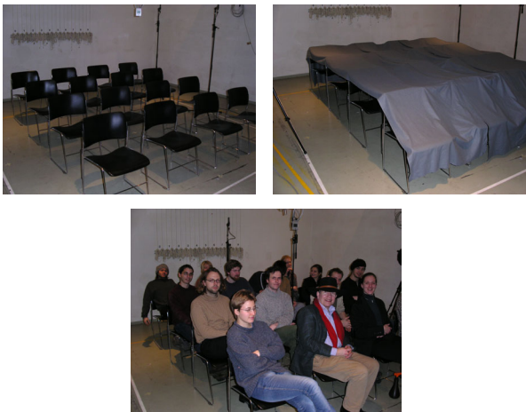
Figure 4: Reverberation chamber of the Allgemeine Unfallversicherungsanstalt (AUVA) in Vienna: unoccupied, with Molton and occupied.
