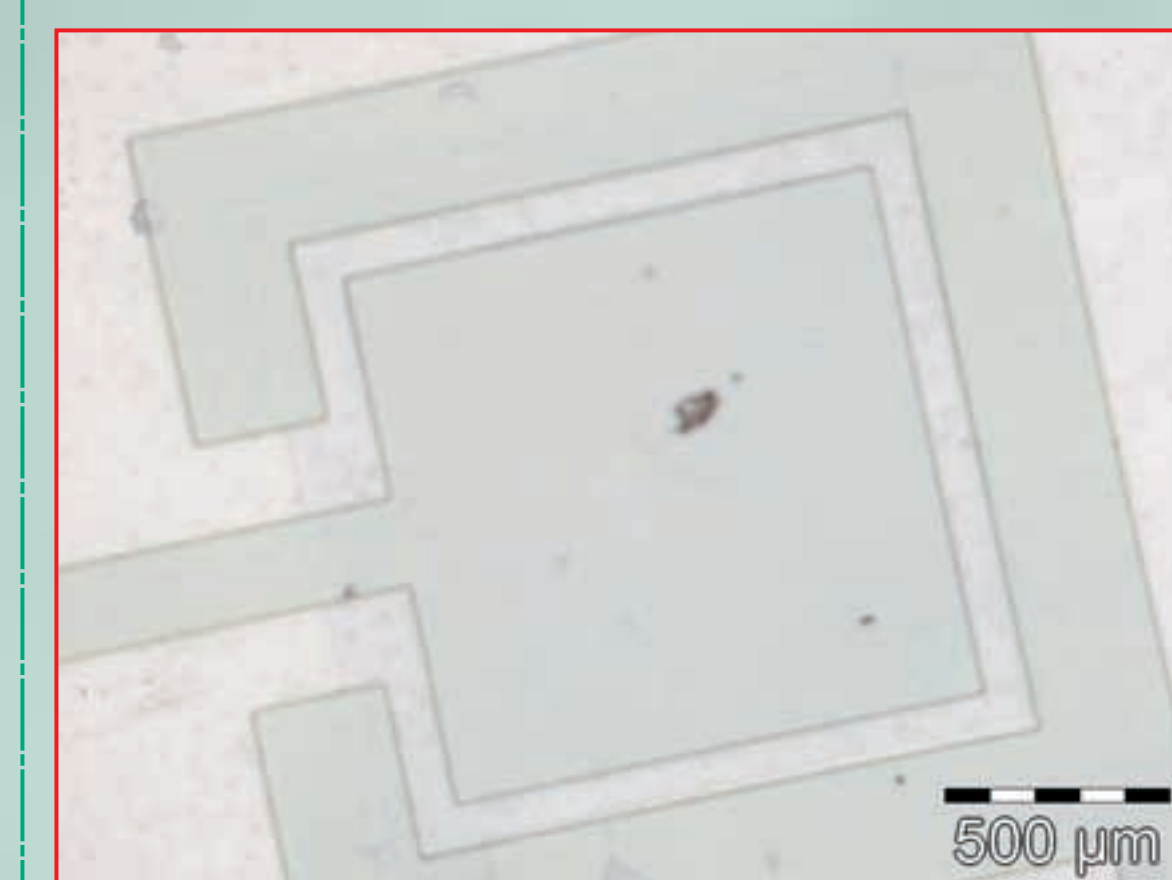
Figure 17: Photograph of aligned source/drain and gate contacts made of Polyaniline, PMMA as dielectric.
