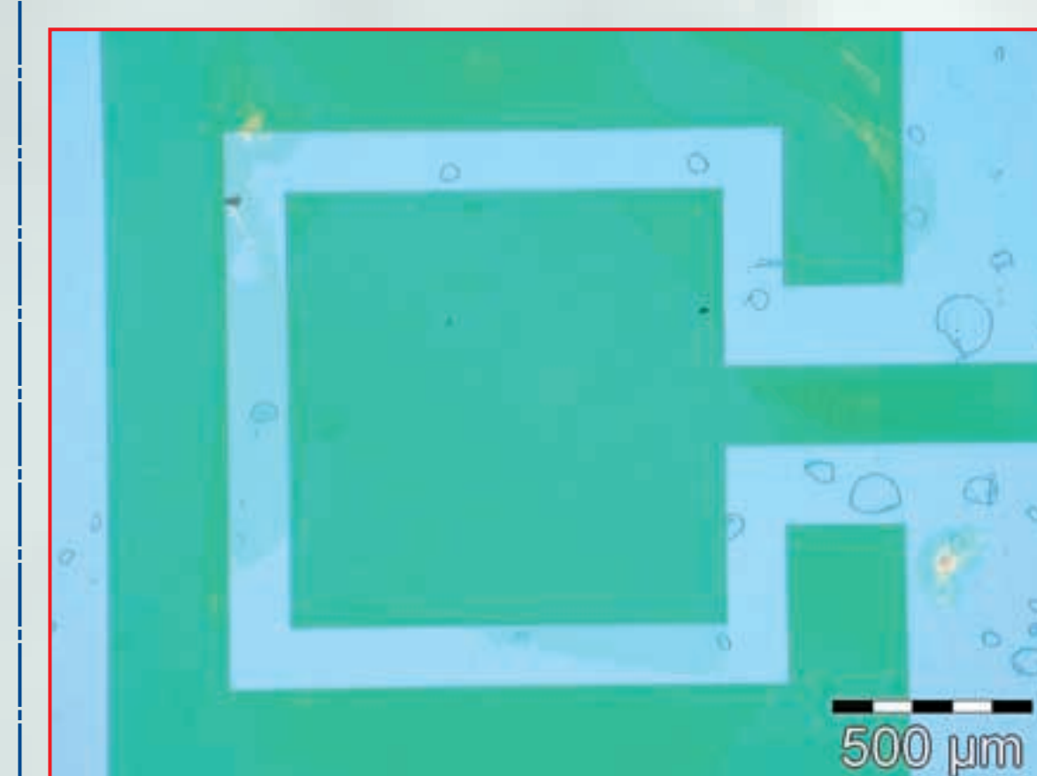
Figure 8: Photograph of photolithographically structured source/drain contacts made of polyaniline on \text{SiO}_2
