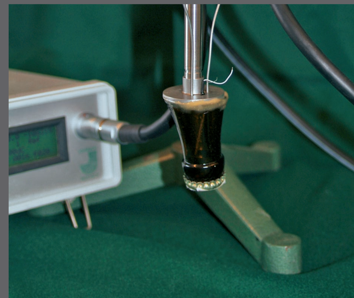
Figure 3: Picture of the measurement set-up to determine the oxygen diffusion through crown caps.
