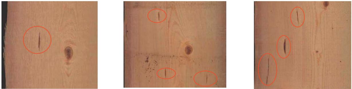
Figures 2a, 2b and 2c: Example of resin pockets on the board surfaces after the cut.
