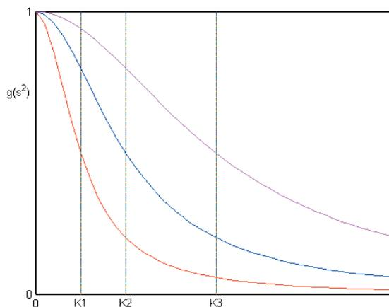
Figure 1: Diffusion parameter as a function of the image gradient.
