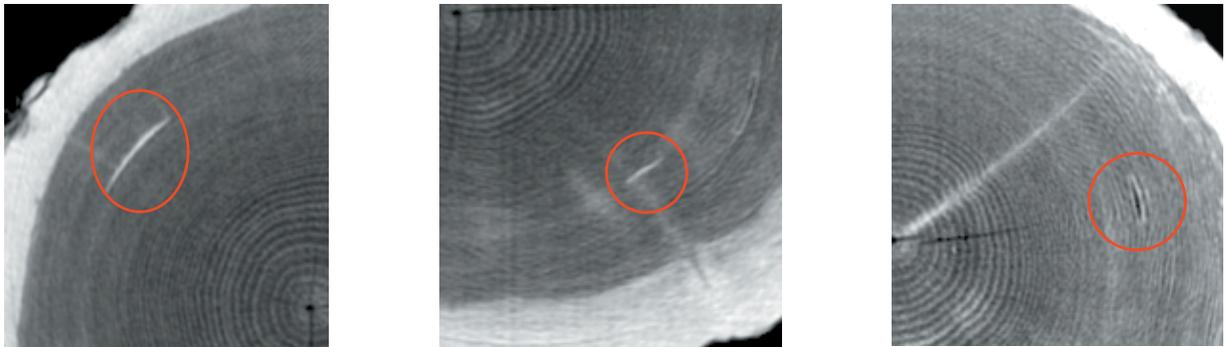
Figures 3a, 3b and 3c: Examples of resin pockets in CT images.
