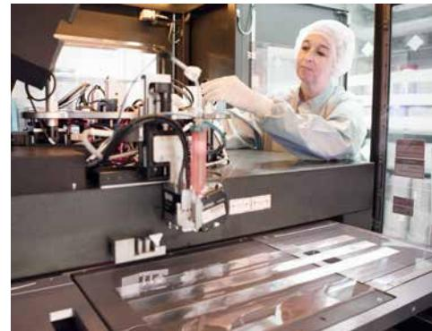
MATERIALS uses a specially modified EVG770 nanoimprint lithography (NIL) stepper for the production of flexible embossing tools for roller-based NIL in the fields of photonics, functional surfaces and microfluidic systems.
