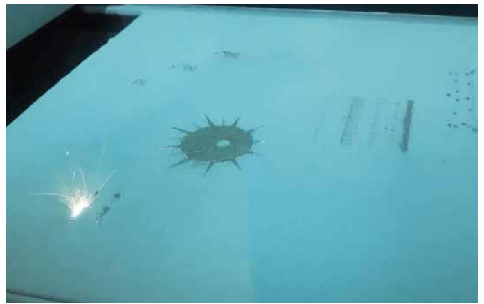
Principle of L-PBF technology (Modified by Materialgeezza - Own work, CC BY-SA 3.0) and Photo of the L-PBF process.
