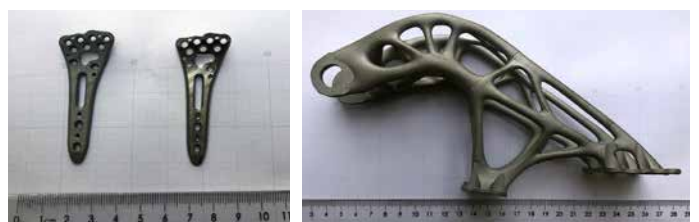
Case examples from medical engineering and aerospace industries (left: bone implants, right: engine maintenance door hinge, both made of titanium)
