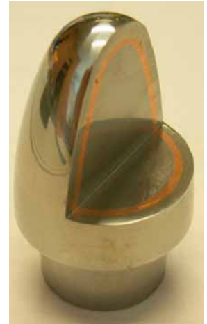
Principle of L-DED technology and additively manufactured component made up of different materials.
