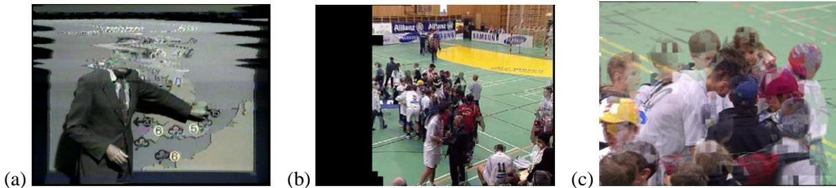
Figure 1: Some typical examples for video breakup impairments caused by analogue (a) and digital (b, c) sources.
