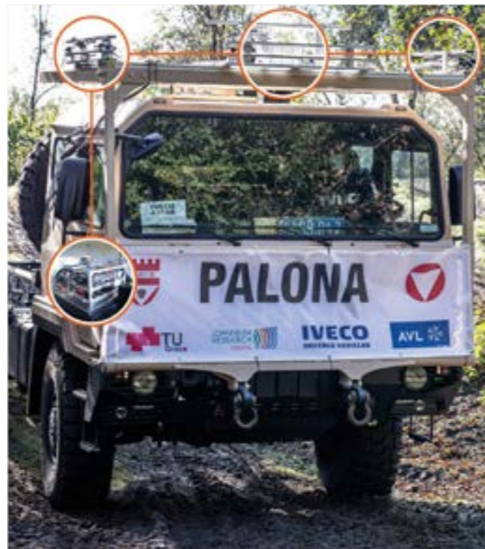
The project resulted in a versatile, mobile sensor system consisting of 8 cameras, an inertial measurement unit (IMU), and a mobile computer. Tests were carried out on military training grounds.
