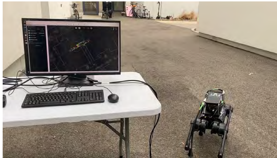
Demo Video: ViFWare/Autoware on Unitree Go1 (Cables only for Monitor/Keyboard)
