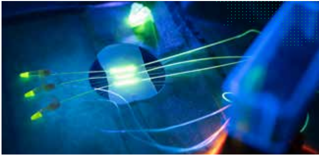
Open flow microperfusion (OFM) enables the continuous collection of interstitial fluid (ISF) in (pre)clinical studies for drug development and biomarker research. Photo: Bergmann
