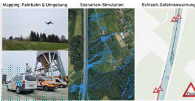
High-precision simulations allow road operators to identify potential bottlenecks in road drainage and to derive preventive infrastructure measures. Photo: JOANNEUM RESEARCH
