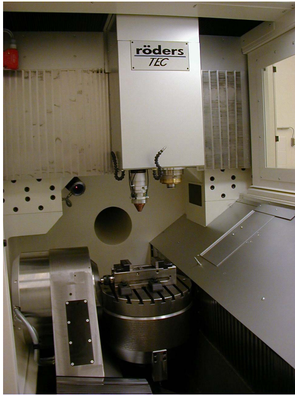
Fig. 5. HSC milling machine combined with a Nd:YAG laser cladding nozzle.
