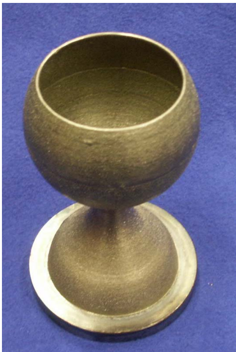
Fig. 19. Wineglass fabricated by 5-axis LC
