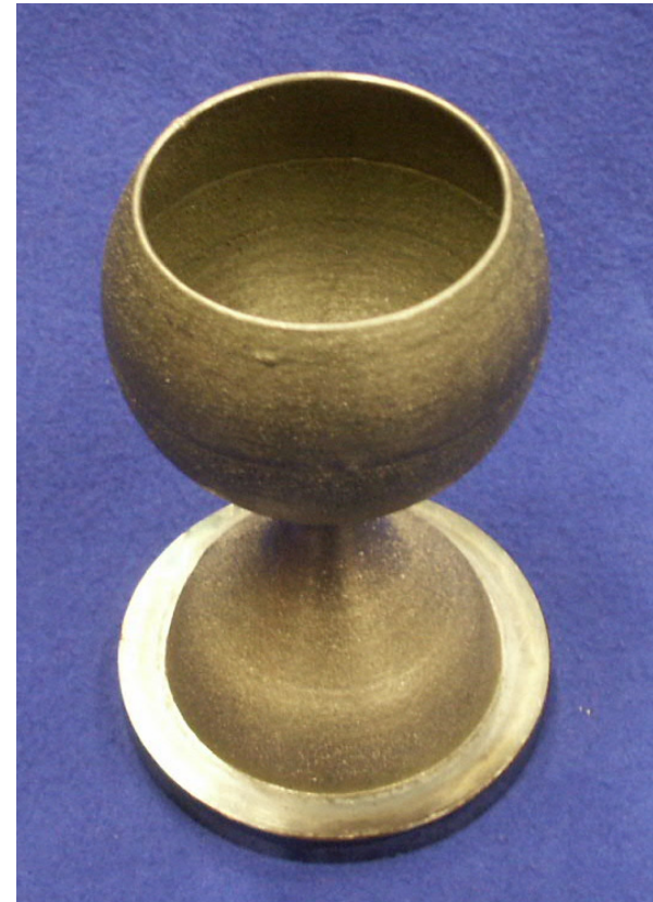
Fig. 17: Wineglass fabricated by 5-axis LC
