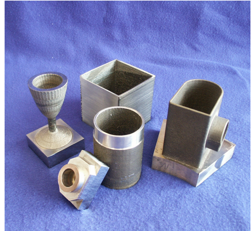
Fig. 16: Nickel-base alloy parts fabricated by 3-axis LC
