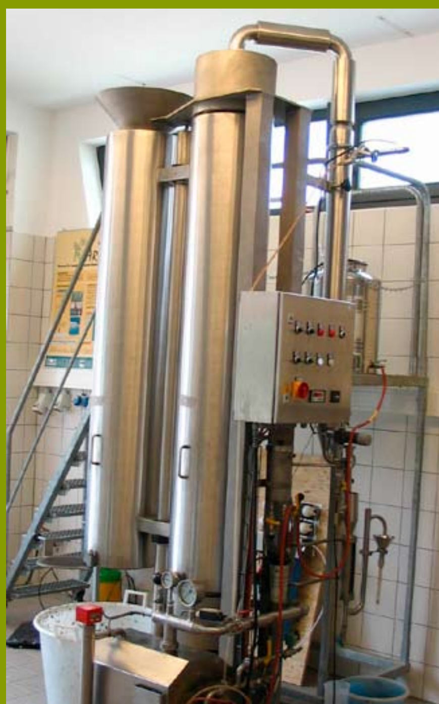
Figure 3: Steam distillation apparatus in pilot plant scale (Herba-Tec, TWE 250-2000)
